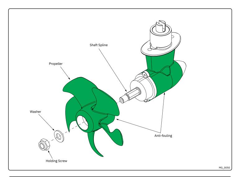
Propeller Installation MC\_0017
