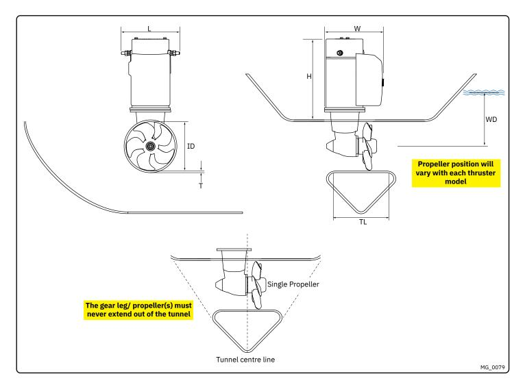
Thruster Measurements MC\_0121
