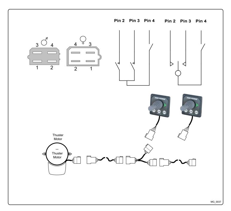
Control Panel Cable Installation MC\_0041
