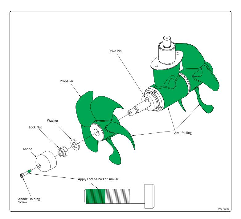
Propeller Installation MC\_0018
