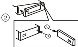
1. Attach the panel at the right side first, with point B on the main unit touching point A on the D.C.P. (As shown on the diagram).
