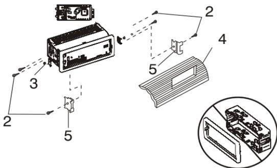
1. Select a position where the screw holes of the bracket and the screw holes of the main unit become aligned (are fitted) and tighten the screws at 2 places on each side.
